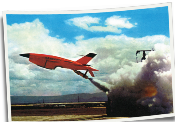
A Ryan Q-2C target missile being launched from a ground station with rocket assist.
